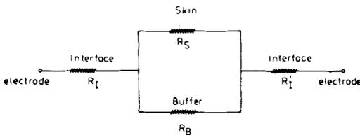
FIG. 3. Electrical model of existing resistances between the electrodes. The  $R_1$  and  $R_2$  are equal and represent the resistances of the interface between electrode and buffer medium containing the skin.  $R_S$  and  $R_B$  are the individual resistances of the skin and the buffer medium ( $R_1$  and  $R_2 \gg R_B$ ), respectively.
